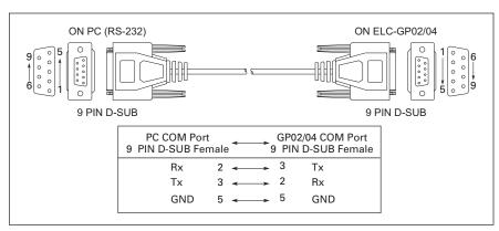
Figure 2. PC to ELC-GPxx Cable
